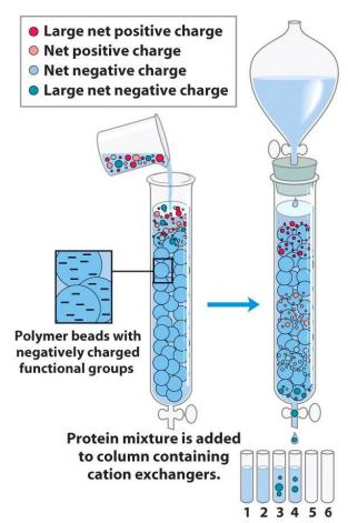
Proteins move through the column at rates determined by their net charge at the pH being used. With cation exchangers, proteins with a more negative net charge move faster and elute earlier.
